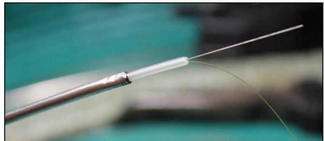
The system is based on the Distributed Temperature Sensing (DTS) technology. A reading unit constantly launches a high frequency light pulse of a specific wave length into an optical fiber and analyses the variations in the so-called Raman frequency in the backscattered spectrum.
